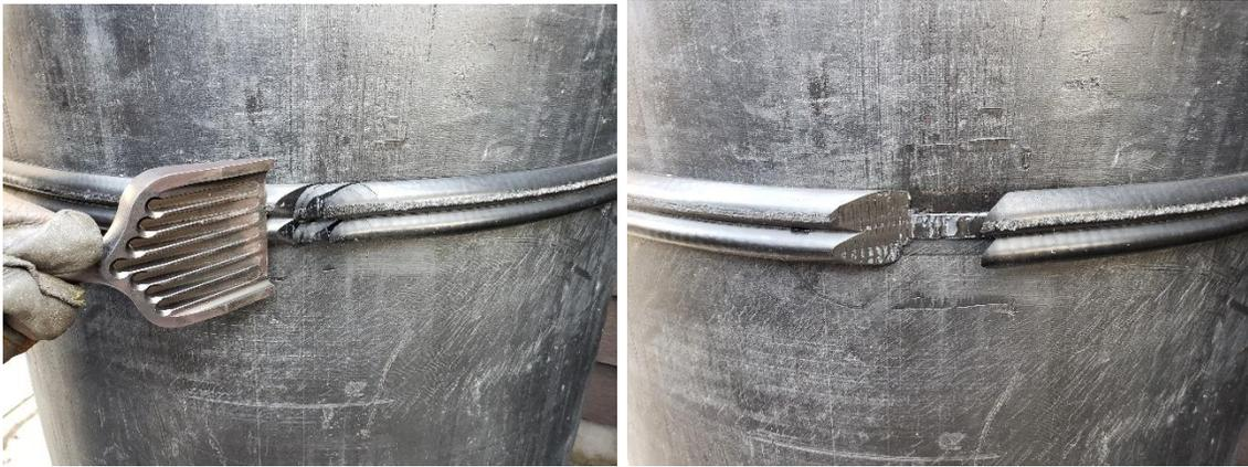
3. After the notch is completed, start the removal operation. On large beads it helps to pull back the bead as you cut away at the root.
