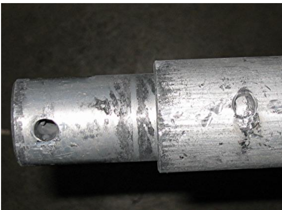
Connector and Torque Tube that has been stressed and deformed
